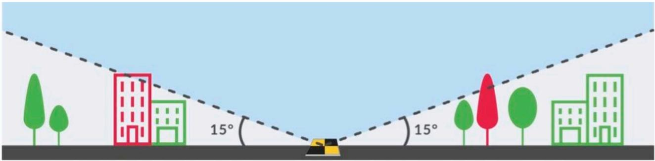
**Important:** AeroPoints (and/or AeroStencil marks) should have an unobstructed view of the sky in every direction above a 15° angle.
